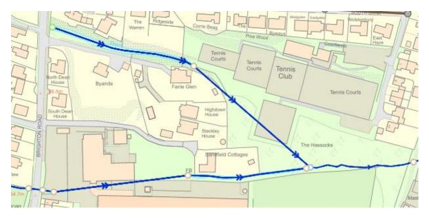
There are historic records of flooding occurring on this site and in this area. The Mid Sussex Strategic Flood Risk Assessment identifies a single flood event in November 2000 at Byanda. This event is classified as fluvial and resulted in internal flooding of the dwelling to a depth of 1.6m. The single recorded flood event does not mean that further flooding has not occurred on site, instead, that further flooding has just not been reported.
